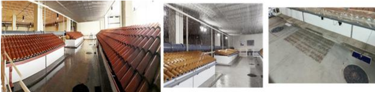
Figure 29: Block Platform for urban drainage and runoff studies at the UDC facilities
