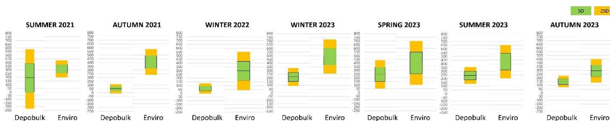
Figure 18: Atmospheric deposition data comparison of sampling campaigns from the 1 st and 2 nd years from Mero-Barcés. Average \pm SD (green) and average \pm 2SD (yellow) of total MP deposition (MP/m 2 /day) encountered for each sampling device in each sampling month ( n = 2 ).
