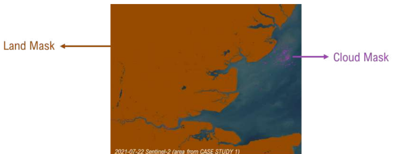
Figure 12 - Masks applied to a LabPlas case study 1 scene in 22-07-2021. Land/water (land in brown and water in transparent) and cloud (clouds in purple) masks are overlapped to a RGB Sentinel-2 image.
